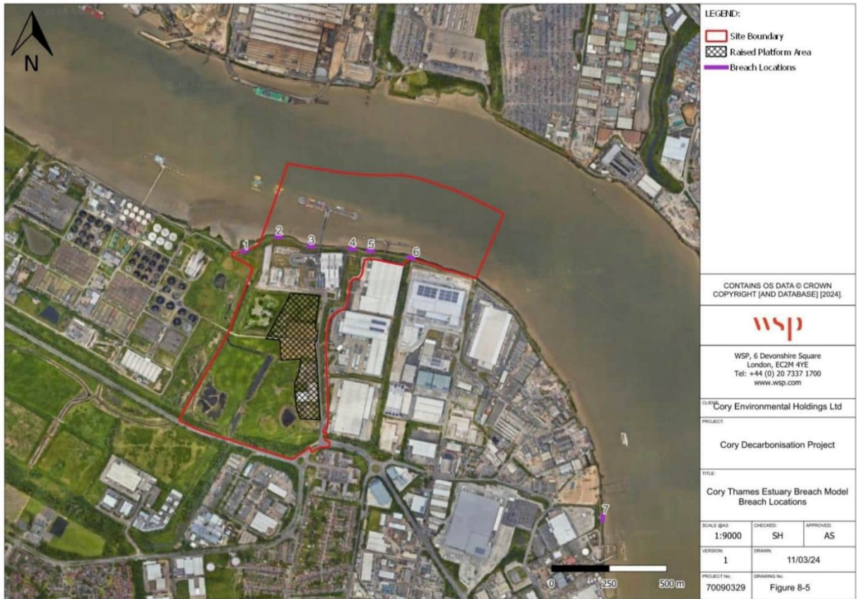
Figure 8-5: Cory Thames Estuary Breach Model Breach Locations
